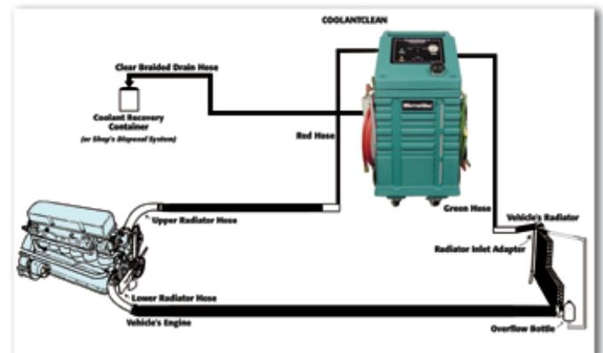
The flush and lubricant process starts from the radiator through all the cooling systems fluid lines and into the water pump.
